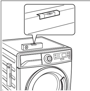
If you do not have a spirit level, as a guide use the edge of a door frame, cupboard or bench to check that the washing machine is level.
