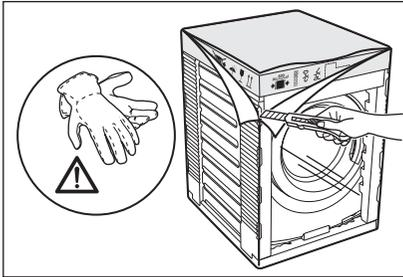
1. Use gloves. Remove the external film. If necessary, use a cutter.
