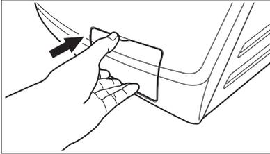
11. Put the flap back and close the drain pump door.
