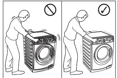
Never place cardboard, wood or similar materials under the machine to compensate for any unevenness in the floor.
