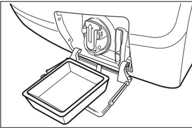
3. Put a container below the recess of the drain pump to collect the water that flows out.
