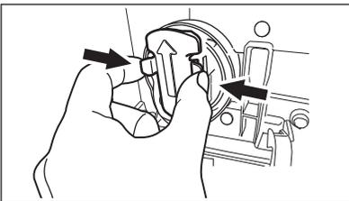
4. Press the two levers and pull forward the drainage duct to let the water flow out.
