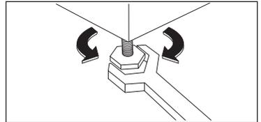
When the washing machine is levelled, try to rock it from corner to corner. If it does rock, adjust the legs again until it is levelled and does not rock.
