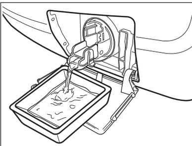
5. When the container is full of water, put the drainage duct back again and empty the container. Do steps 4 and 5 again and again until no more water flows out from the drain pump.
