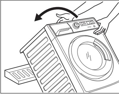
6. Put one of the polystyrene packaging elements on the floor behind the appliance. Carefully put down the appliance with the rear side on it. Make sure not to damage the hoses.
