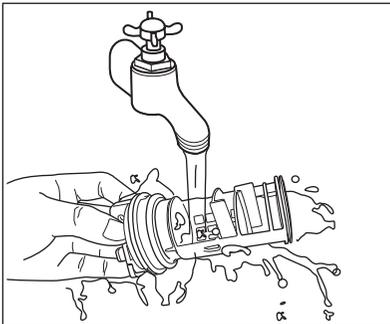
6. Pull back the drainage duct and turn the filter to remove it.
