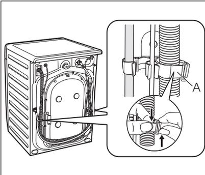
9. Remove the power supply cable and the drain and inlet hoses from the hose holders (A) on the rear of the appliance.
