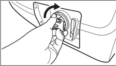
10. Put the filter back in the pump into the special guides. Make sure that you tighten correctly the filter to prevent leakages.
