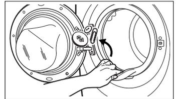
Check and remove objects (if there are any) that could be trapped in the fold.
