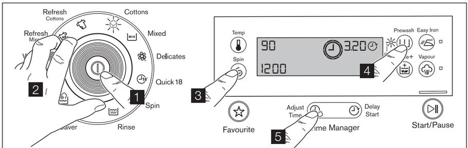
1. Press the On/Off button to turn on the washing machine.
