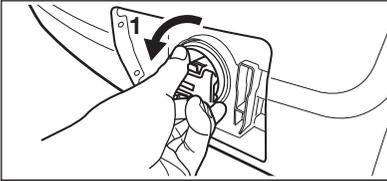
6. Pull back the drainage duct and turn the filter to remove it.
