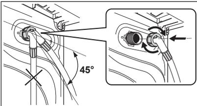
6. Install again the inlet hose. Make sure that the couplings are tight to prevent leakages.
