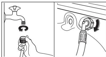
The inlet hose must not be lengthened. If it is too short and you do not wish to move the tap, you will have to purchase a new, longer hose specially designed for this type of use.
