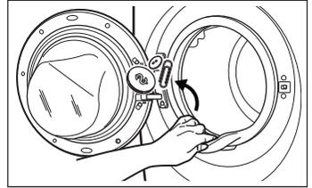
Check and remove objects (if there are any) that could be trapped in the fold.
