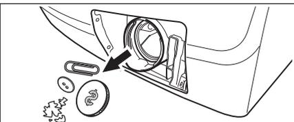
7. Make sure that the impeller of the pump can turn. If this does not occur, contact the service centre.
