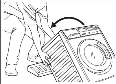
6. Put one of the polystyrene packaging elements on the floor behind the appliance. Carefully put down the appliance with the rear side on it. Make sure not to damage the hoses.
