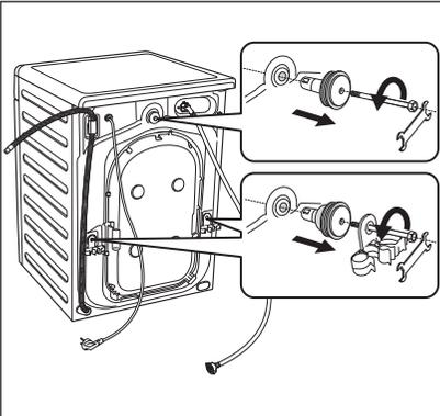
10. Remove the three bolts. Use the key supplied with the appliance.
