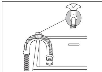
In this case, make sure the end cannot come unhooked when the machine is emptying.
