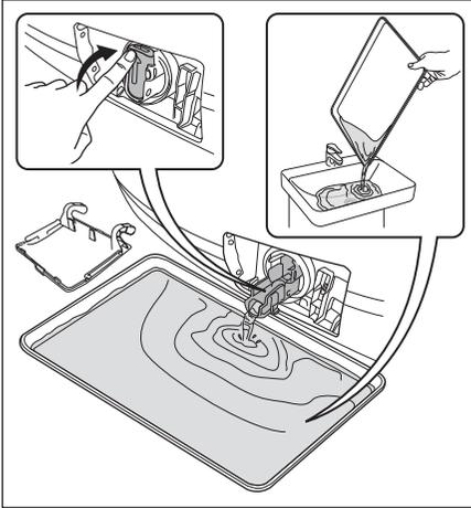
5. Pull back the drainage duct and turn the filter anti-clockwise to remove it.
