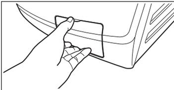
2. Pull the flap down, then squeeze the legs on both sides of the cover together and pull out (as picture).
