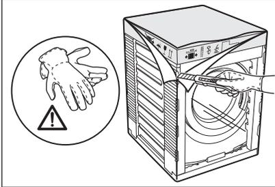
1. Use gloves. Remove the external film. If necessary, use a cutter.
