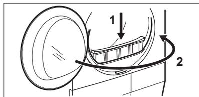
1) If necessary clean the filter with tap warm water using a brush and/or a vacuum cleaner.
