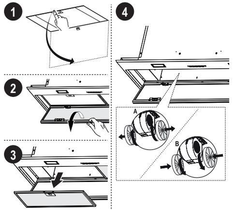
The carbon filter must always be used if the cooker hood is not ducted.
