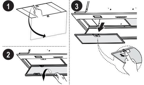
Switch off the electricity! Remove the plug from the socket or switch the electricity off at the mains. Open the panel and pull the special handle to remove the filter.
