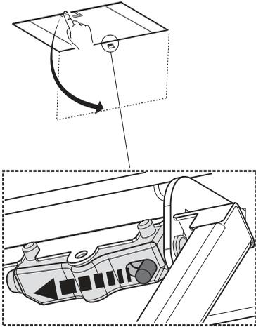
2. Remove the grease filter.
